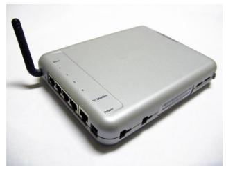
your broadband modem through an Ethernet cable. The wireless router transmits a signal to the built-in wireless receiver in the laptop, giving you increased mobility with the laptop at home.
